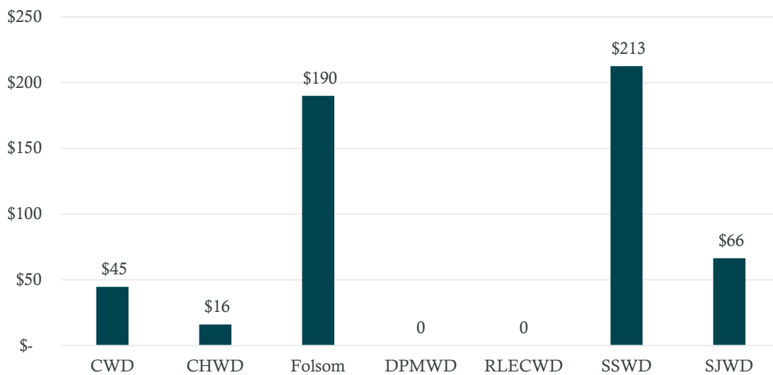
Figure 6: Leak Detection Costs per Mile of Pipe 13
