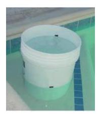
Leave the bucket in the pool undisturbed for several warm days, then compare the water level in the bucket to the level in the pool.
